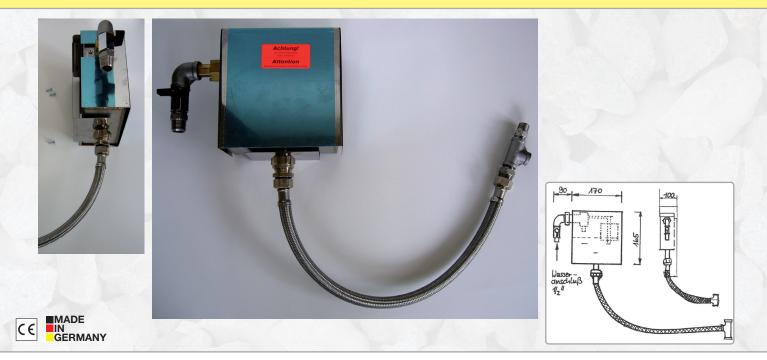
Automatic water-refill of the vaporizer by a servo-controlled mechanical float-valve in a external refill-box by the local water connection.
