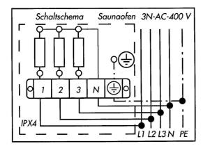
The connection diagram for the room heating section of the sauna heater is attached at the inside of the oven back panel and corresponds to the illustration opposite.
