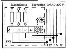
The connection diagram for the room heating section of the sauna heater is attached at the inside of the oven back panel and corresponds to the illustration beside.
