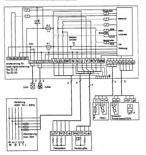
If the system is operated with a control unit without lack of water, the Terminal "WM" in control unit unused!
