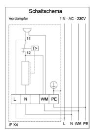
The connection diagram for the vaporizer (Wall-steamer) corresponds to the illustration beside.
