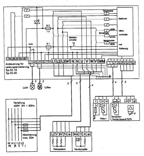
If the system is operated with a control unit without lack of water, the Terminal "WM" in control unit unused!
