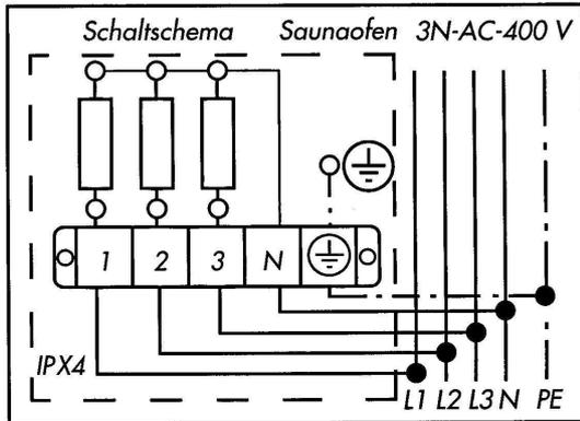
The connection diagram for the room heating section of the sauna heater is attached at the inside of the oven back panel and corresponds to the illustration opposite.
